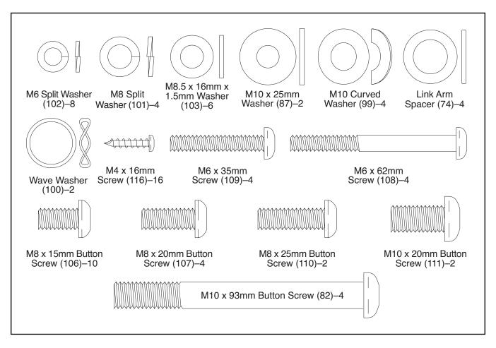
1. While another person lifts the front of the Frame (1), attach the Front Stabilizer (4) to the Frame with two M10 x 93mm Button Screws (82) and two M10 Curved Washers (99).
